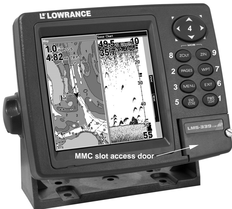
LMS-339cDF iGPS sonar unit showing map with sonar split screen, keyboard and access door for the MMC slot.
